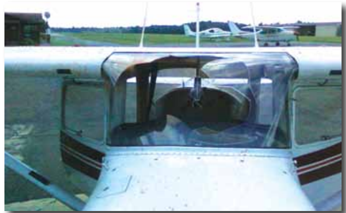
The impact of the turkey vulture destroyed the windshield of the Cessna 152 that Kimberly was piloting.
