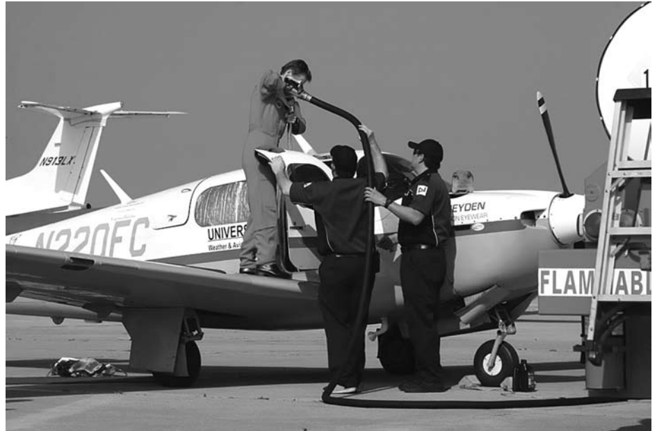
CarolAnn fills the ferry tanks through an extension hose.
