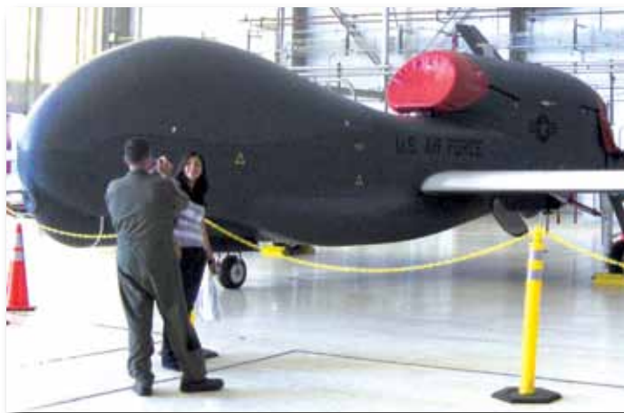
U.S. Air Force Global Hawk, a high-altitude, remotely piloted reconnaissance aircraft.
